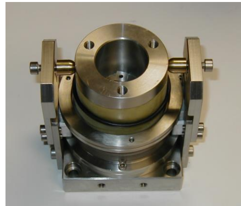
Fig. 9 GDS simple shear sample preparation equipment
