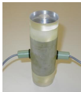
Fig. 4 Horizontal elements mounted to specimen
