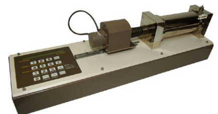
Fig 5. Advanced Pressure Controller used in Unsaturated Testing
