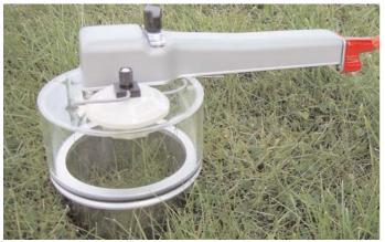
A number of other plant leaf chambers are available for use with the SRS1000 and SRS2000 enabling photosynthesis analysis measurements on a wide variety of plant species.
