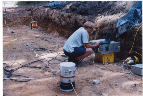
Fig 3. Photograph showing a six-geophone layout on one of our test sites
