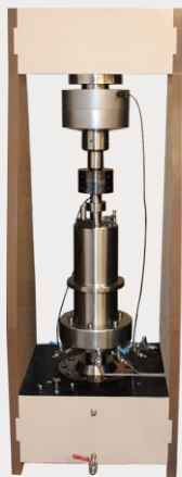
Static Load Frame
