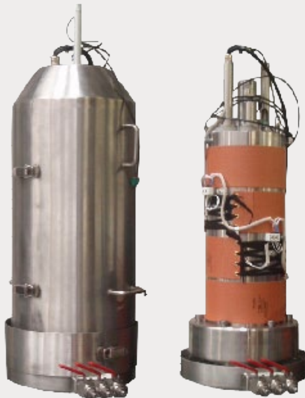
Fig 8. 20MPa high pressure cell with the temperature control.
